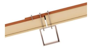
In this way shear stresses are more effectively relieved on the supporting structure via fixing units. This layout is suitable above all for overlapping panels of greater length.
