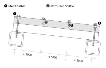
Once the panel is in place, drill the first hole. Remember to use the cap as a template, to center hole on the rib well. Always make sure the hole is perpendicular to the panel surface.
