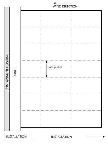
Once the starting point is set and alignments have been checked with respect to the structural work, it is possible to start laying the first roofing panel, **following the intended installation direction**.
