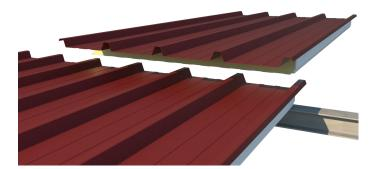
With the first line of panels completed, proceed with the overlapping of the first panel.
