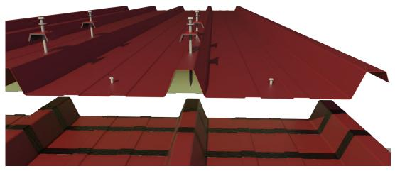
Frontal view of an overlap made using two strips of intumescent sealant placed on the trapezoidal substrate of the underlying panel, two trapezoidal cap screws and stitching screws on the flat side.
