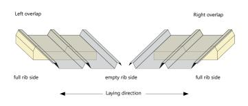
The sheet of the upstream overlapping panel overlaps the downstream panel and is fixed with stitching screws at the ribs so as to avoid deformation and bending of the overlapping sheet.
