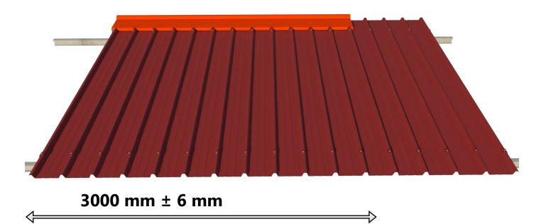
Pay close attention to the right coupling of panels during the installation (3 panels =  $3000 \text{ mm} \pm 6 \text{ mm}$ ) in order to avoid problems during the installation of the roof ridge.
