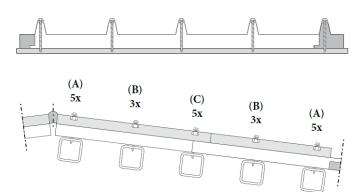
Fix the roofing panel with appropriate screws.
