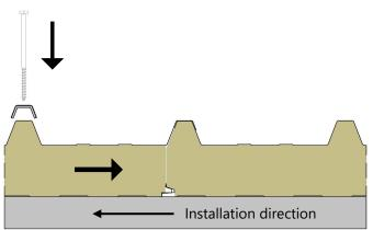
The second panel must be installed overlapping the empty rib on the full rib of the first panel.
